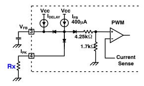
Figure 23. Peak Current Limit Adjustment
