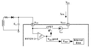
Figure 14. Startup Circuit
