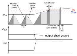
Figure 20. Output Short Waveforms (OSP)
