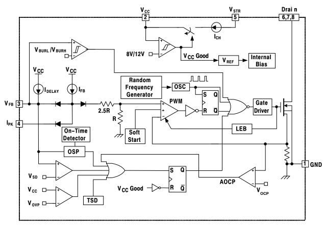
Figure 2. Internal Block Diagram
