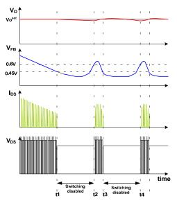
Figure 22. Burst-Mode Operation
