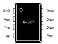
Figure 3. Pin Configuration
