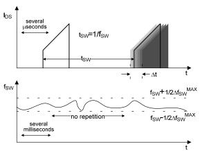
Figure 15. Frequency Fluctuation Waveform
