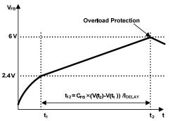
Figure 18. Overload Protection (OLP)
